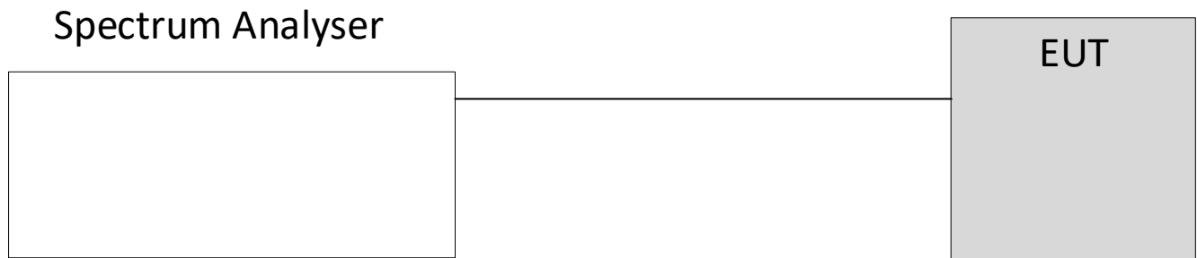
Figure 4.5-2: Antenna port testing block diagram
