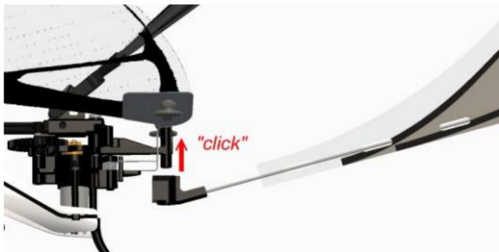
Insert the rudder end by pressing it up on the tube at the end of the steering system, while holding the upper side of this tube with the other hand's forefinger to balance the force. Spread the spring ends if necessary, they must stay outside of the rudder end.
