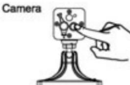
2. Mount the Magnetic Camera on your tailgate, and then adjust it to a suitable angle.
