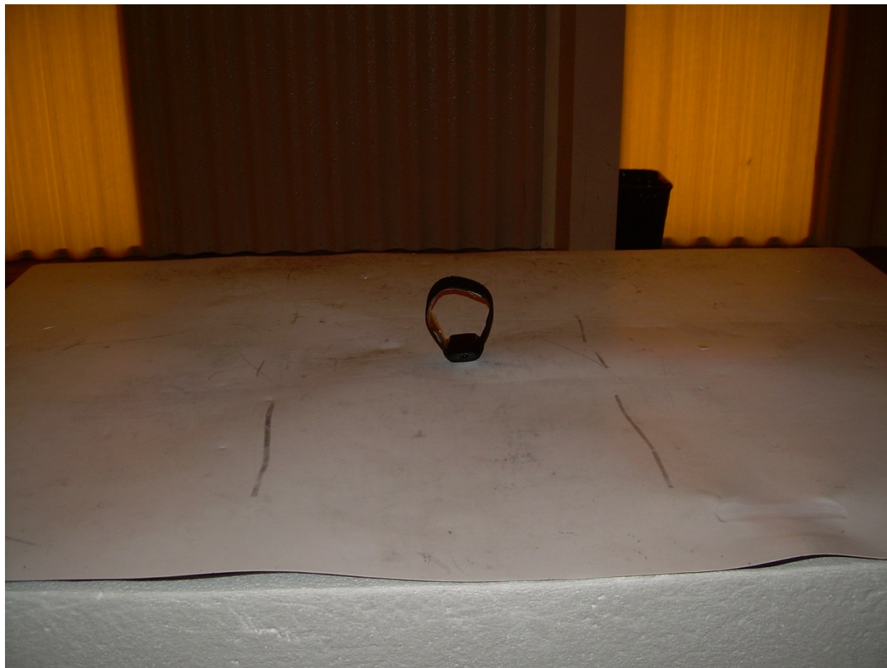
Photograph 1 – Front View Radiated Disturbance Worst Case Configuration – Flat
