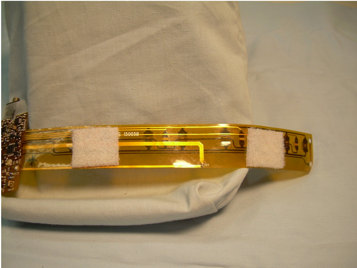
Photograph 11 – View of the Outer Side of the Flex Band and Antenna
