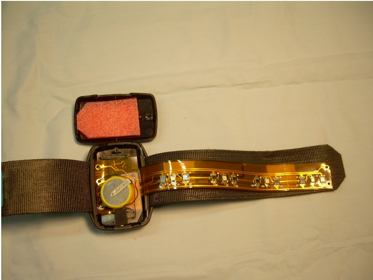
Photograph 7 – View with the XTMR 103 Housing Opened
