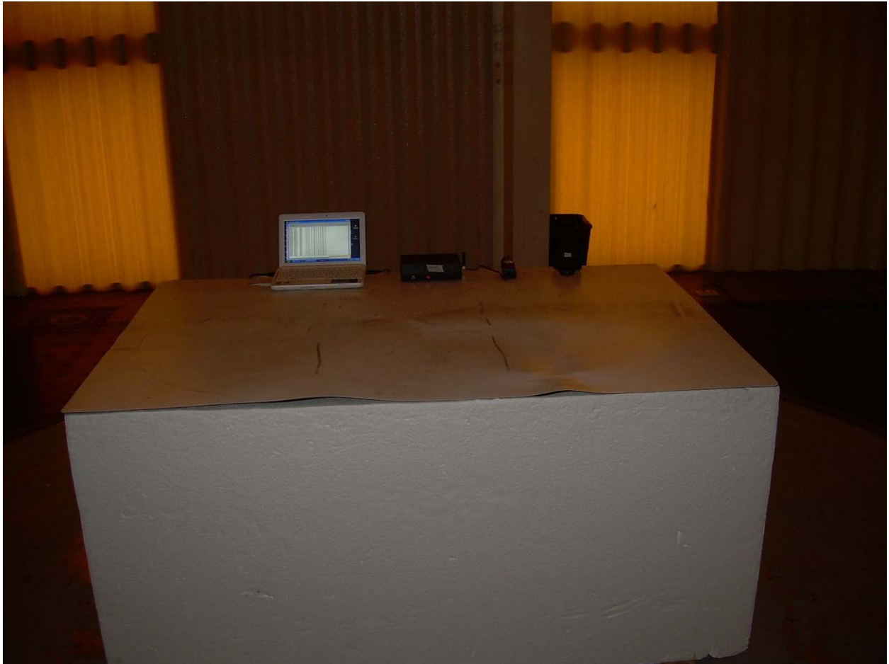
Front View - Radiated Disturbance Worst Case Configuration
