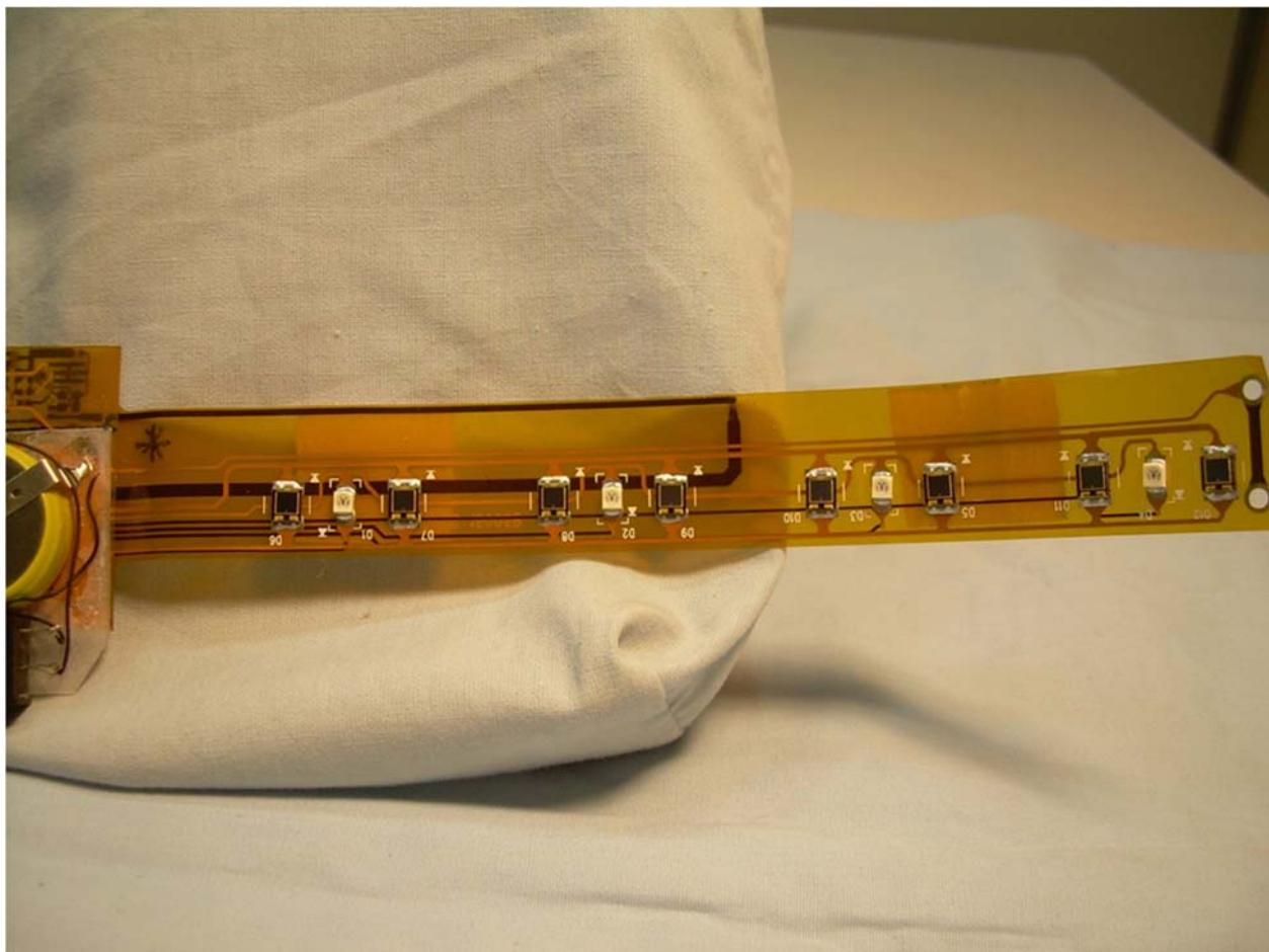
View of the Outer Side of the Flex Band and Antenna
