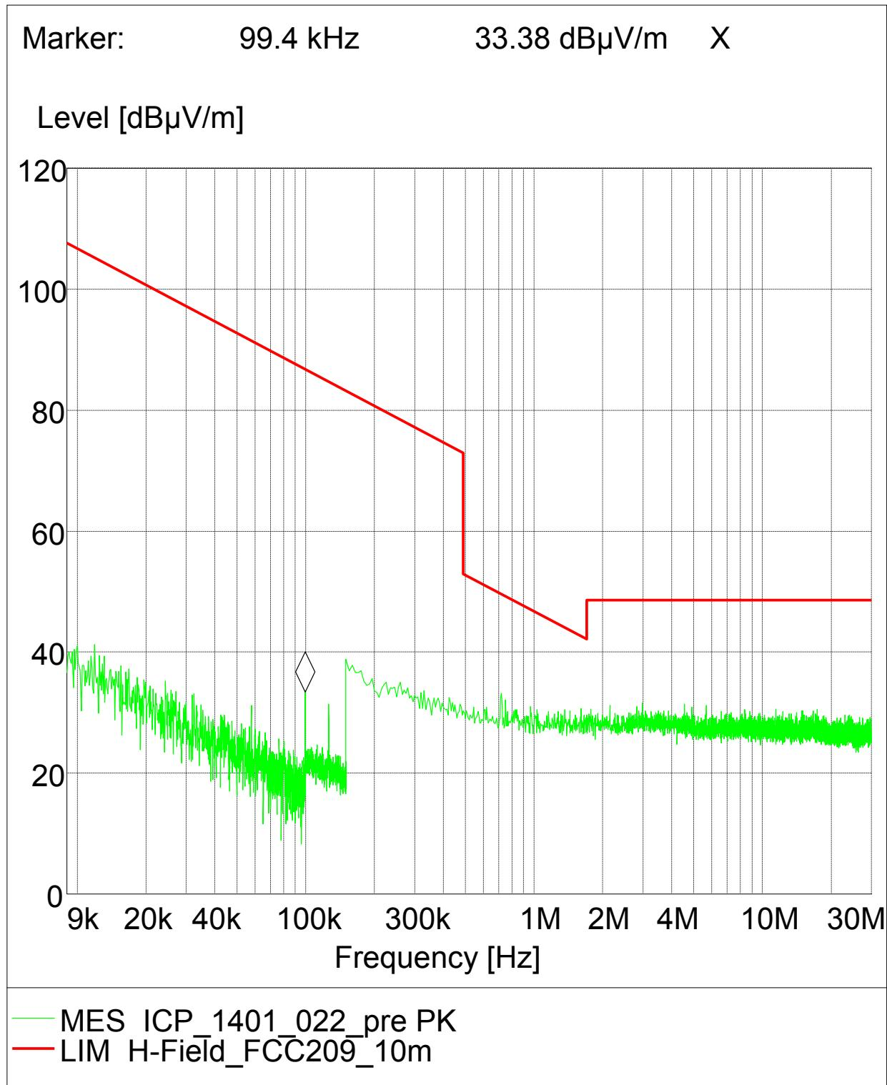
Remark: The peak found at 99.4 kHz is an emission from the loop antenna power supply
