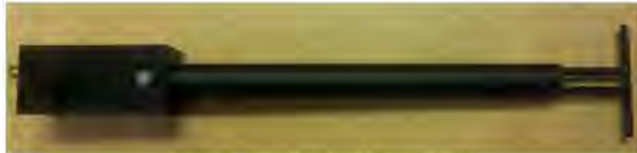
Figure 1 – MVG COMOSAR Validation Dipole
