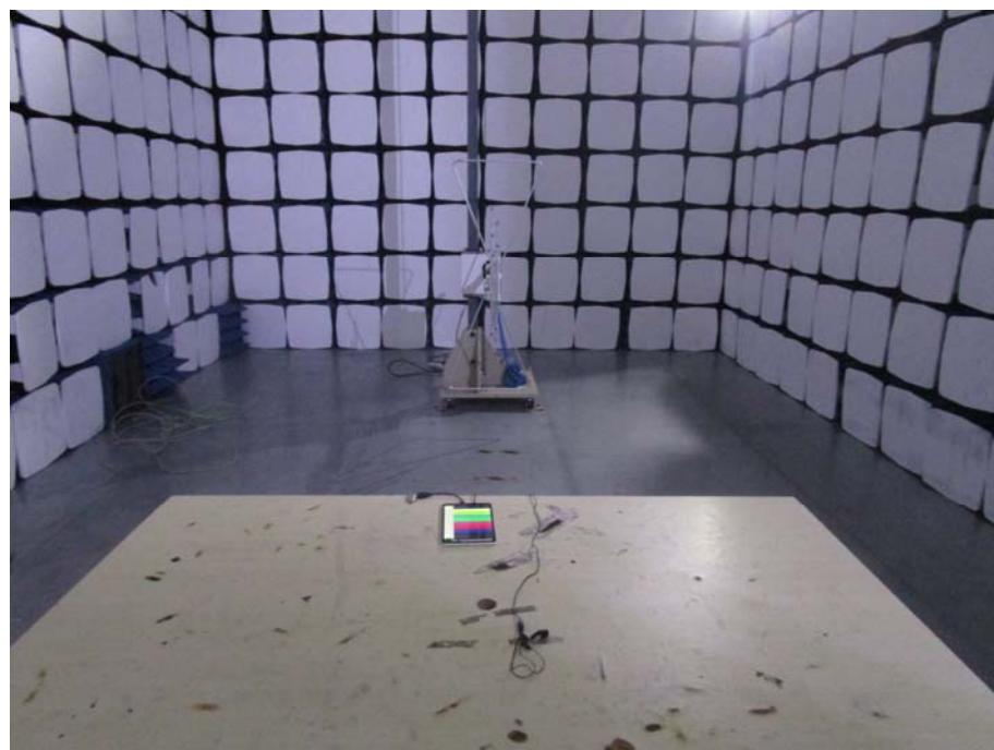
**Radiation Emission Test Setup (Above 1GHz)****Charging And HDMI Playing**
