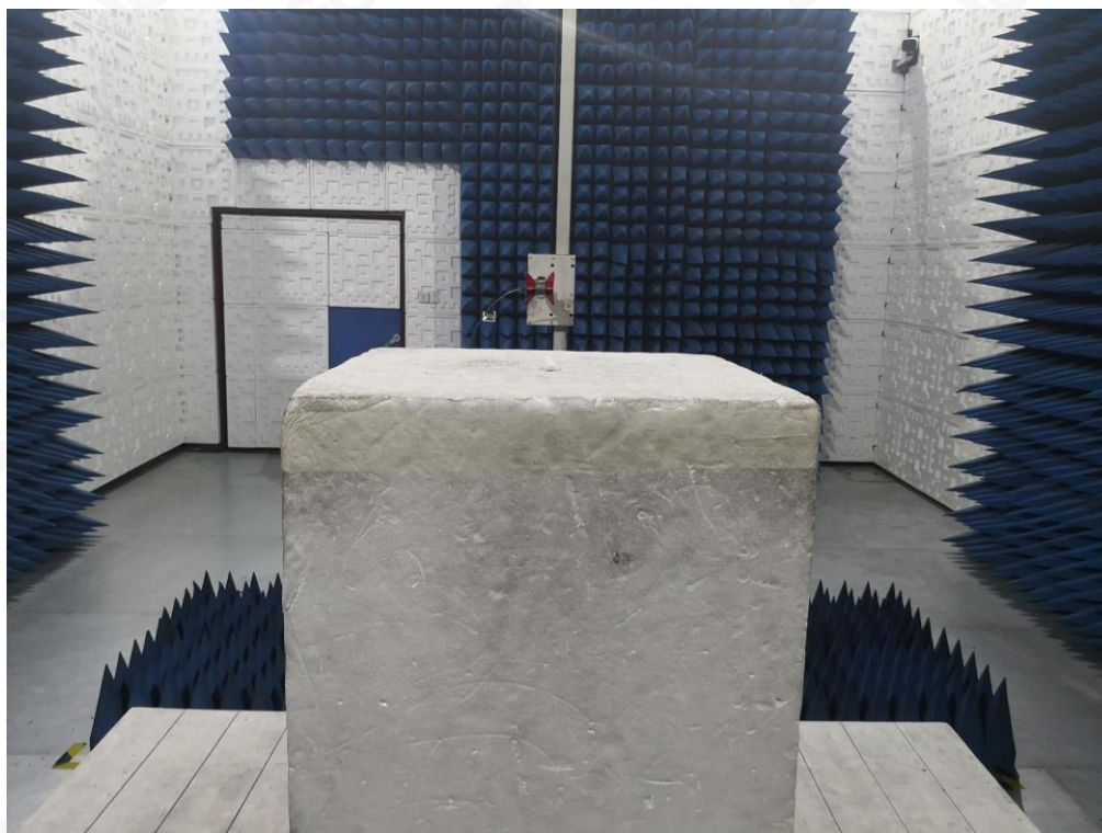
RADIATED EMISSION TEST SETUP ABOVE 1GHZ
