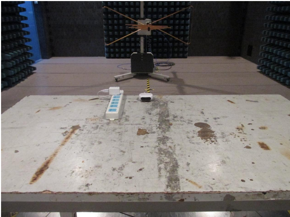
Radiated Emission Test setup photos
