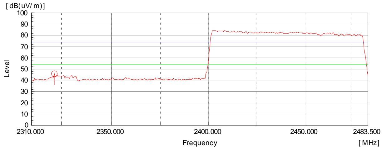
AV Detector: RBW: 1 MHz, VBW: 10 Hz (2 310 MHz - 2 390 MHz), Worst case (Low, Vertical)
