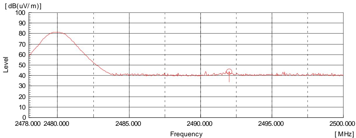
AV Detector: RBW: 1 MHz, VBW: 10 Hz (2 483.5 MHz - 2 500.0 MHz), Worst case (High, Vertical)
