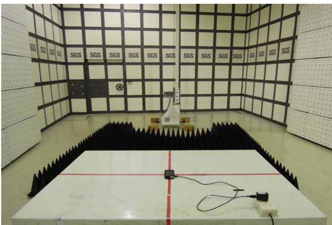
**Radiated Emission Set up Photos (H PLAN Above 1GHz)**
