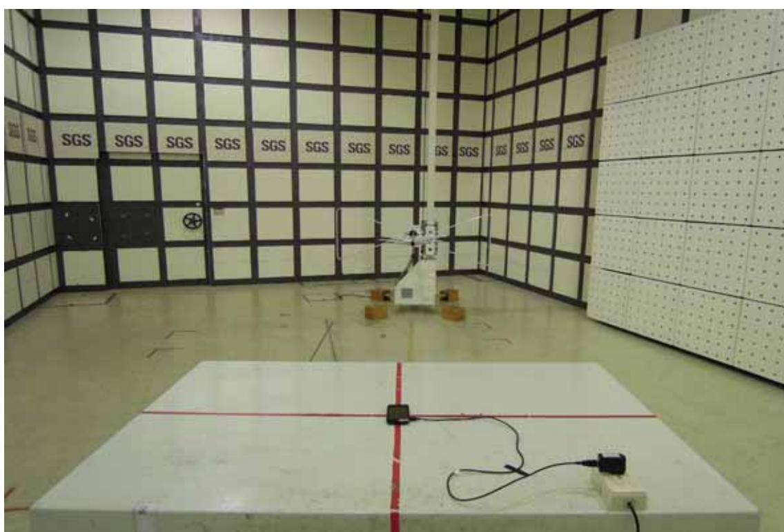
**Radiated Emission Set up Photos (H PLAN Below 1GHz)**
