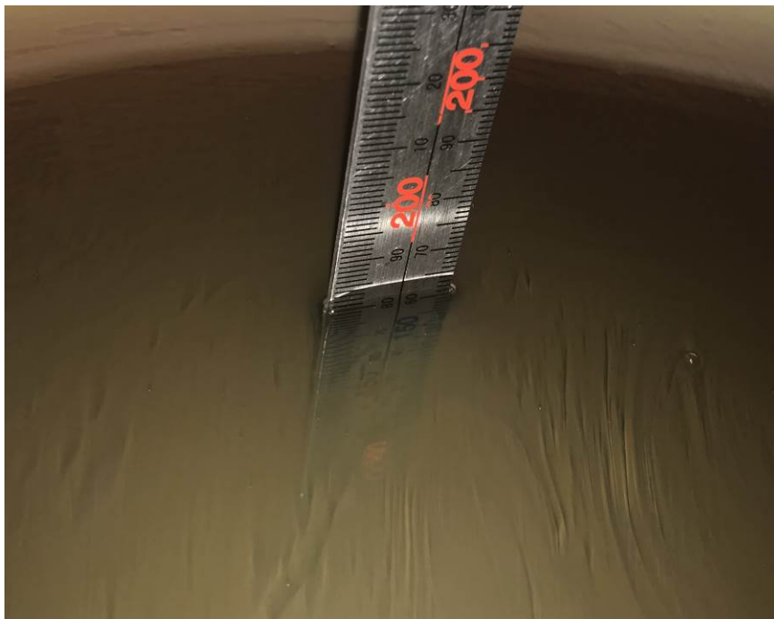
Liquid depth for SAR Measurement
