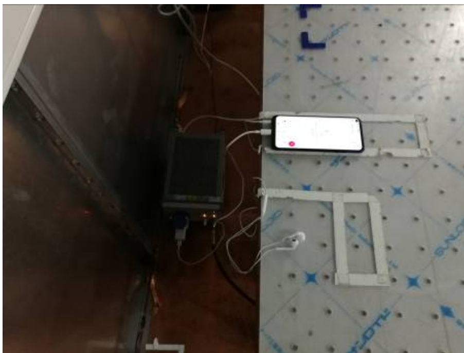
Conducted Emissions Test Setup (with charger)
