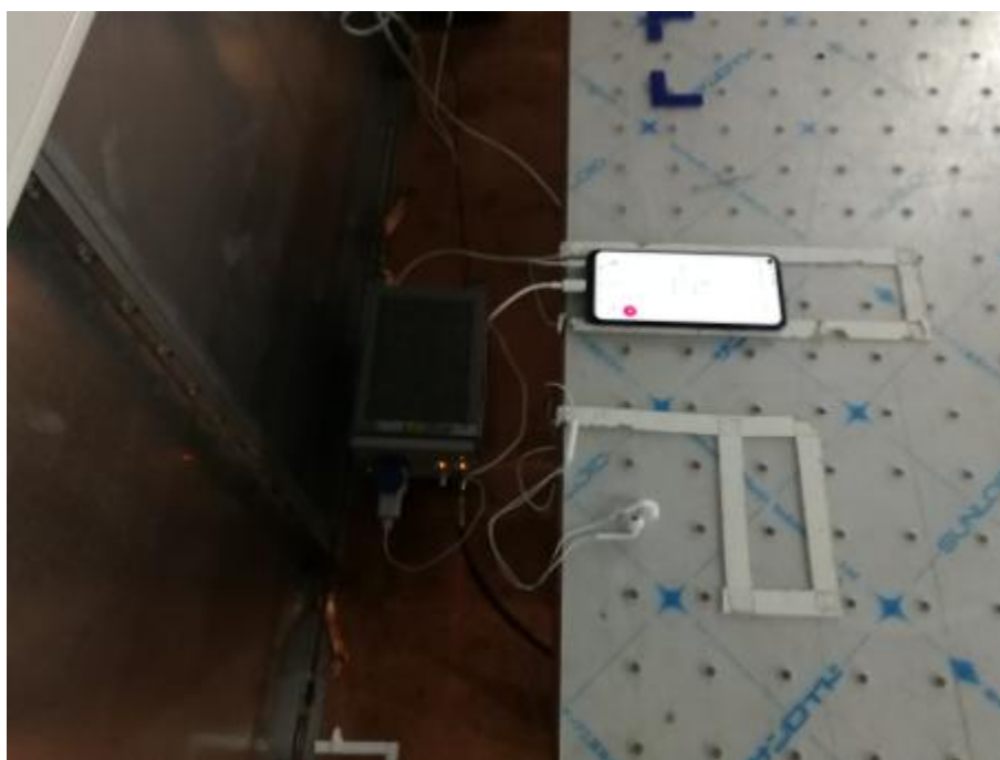
Conducted Emissions Test Setup (with charger)
