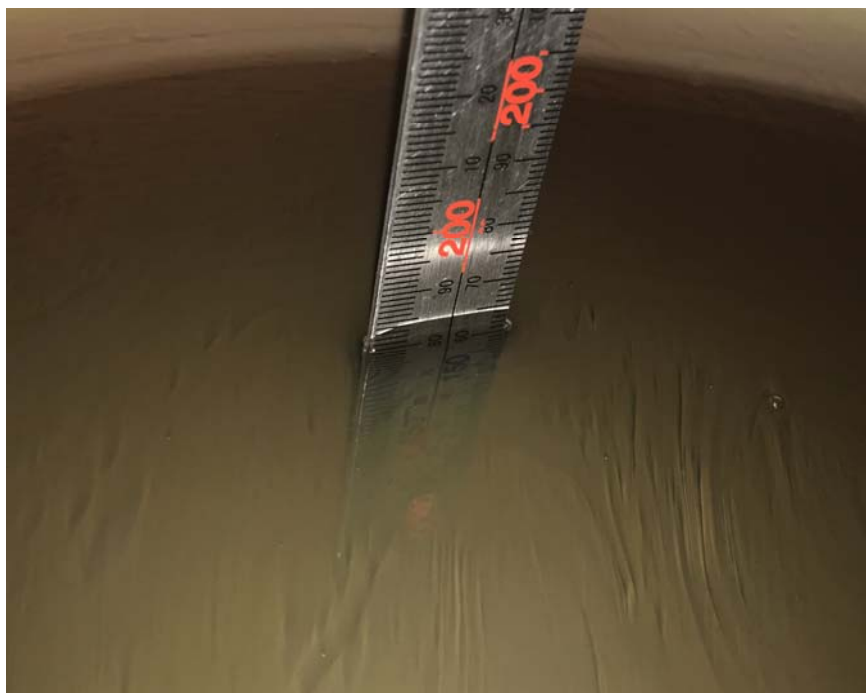
Liquid depth for SAR Measurement
