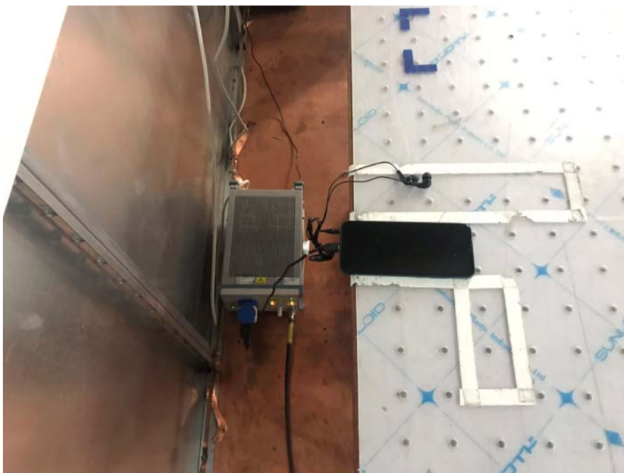
Conducted Emissions Test Setup (with charger)
