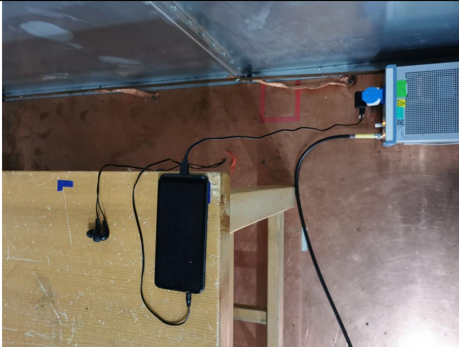
Conducted Emissions Test Setup (with charger)
