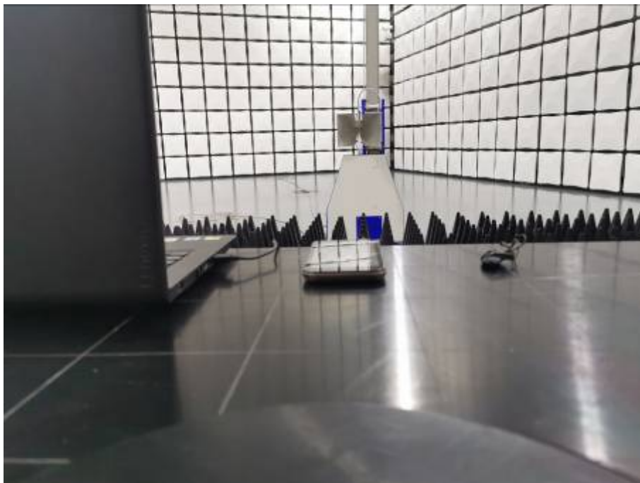
Radiated Emissions Test Setup (above 1GHz)
