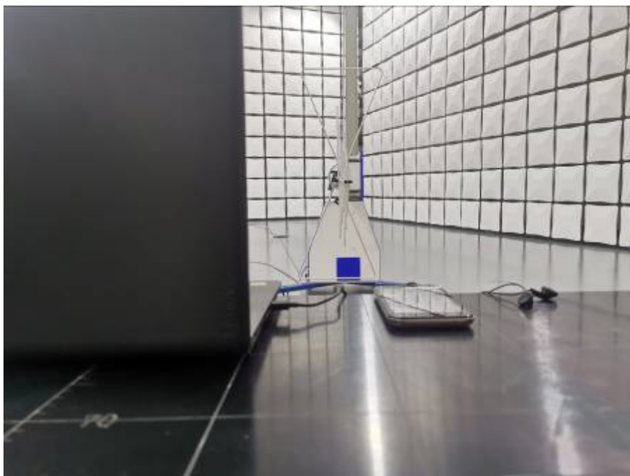
Radiated Emissions Test Setup (30-1000MHz)
