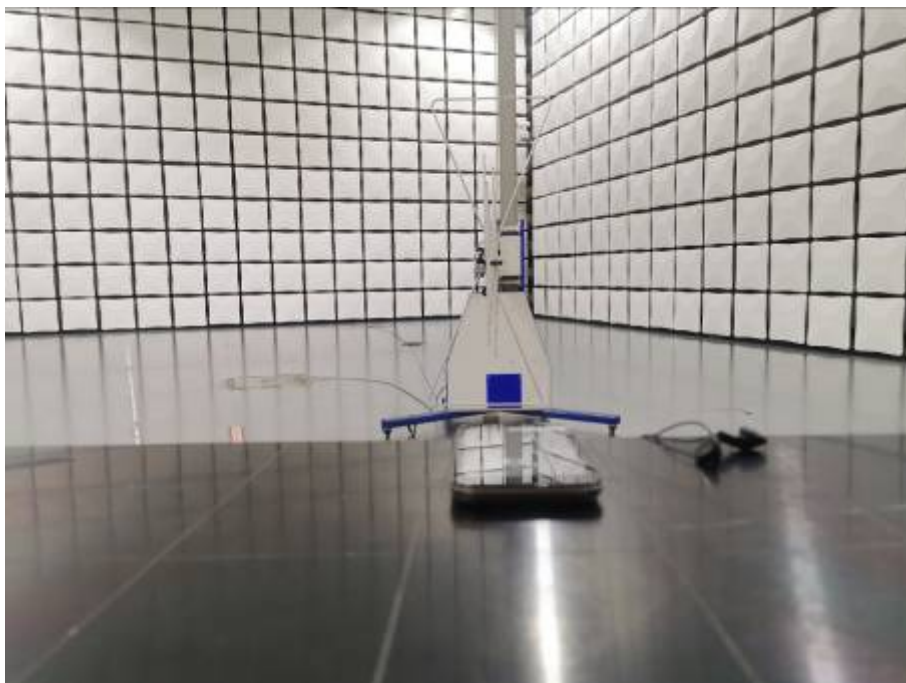
Radiated Emissions Test Setup (30-1000MHz)
