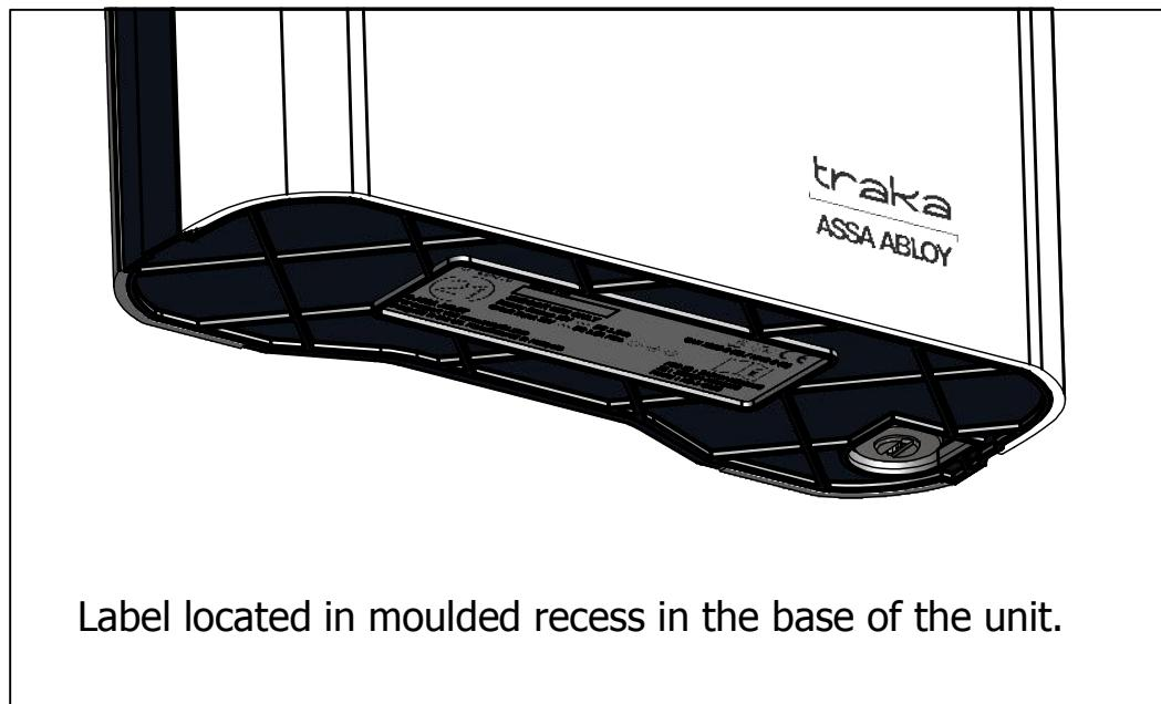
Label located in moulded recess in the base of the unit
