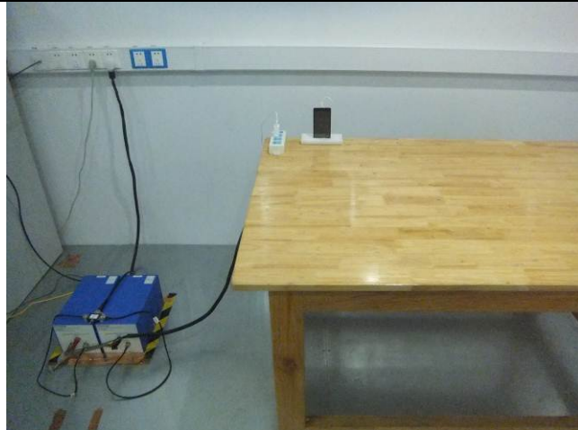
Conducted Emissions Test Setup Front View
