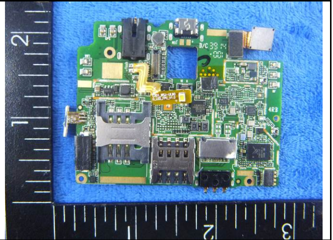
Mainboard Without Shielding - Front View
