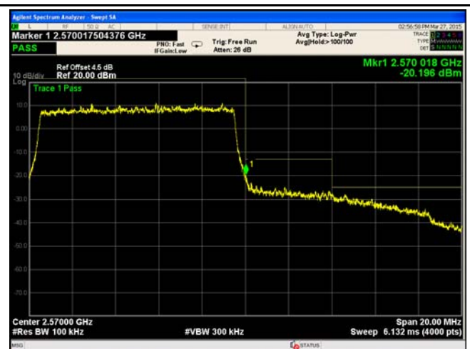
LTE Band 7 - High Channel 16QAM-10
