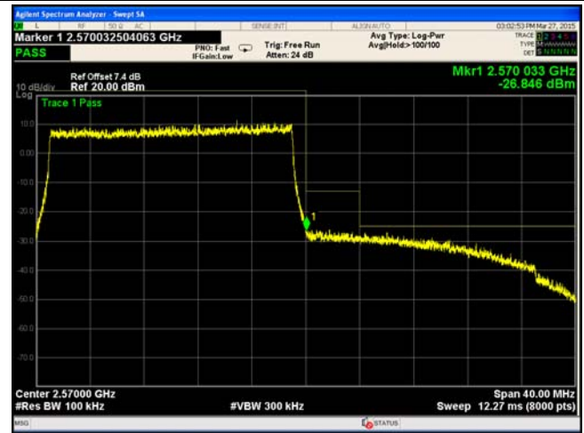
LTE Band 7 - High Channel 16QAM-20
