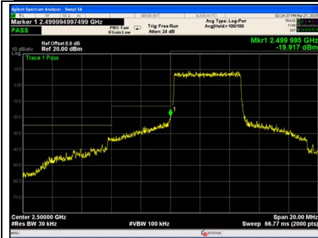
LTE Band 7 - Low Channel 16QAM-5
