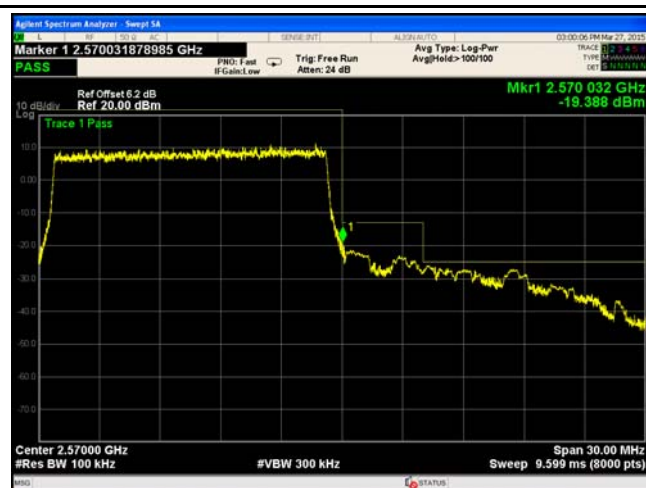
LTE Band 7 - High Channel 16QAM-15
