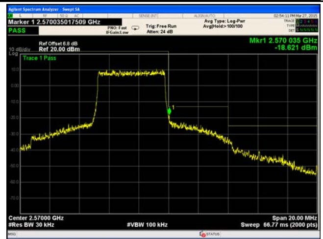
LTE Band 7 - High Channel 16QAM-5
