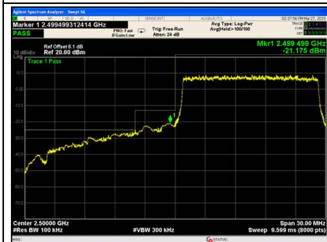
LTE Band 7 - Low Channel 16QAM-15
