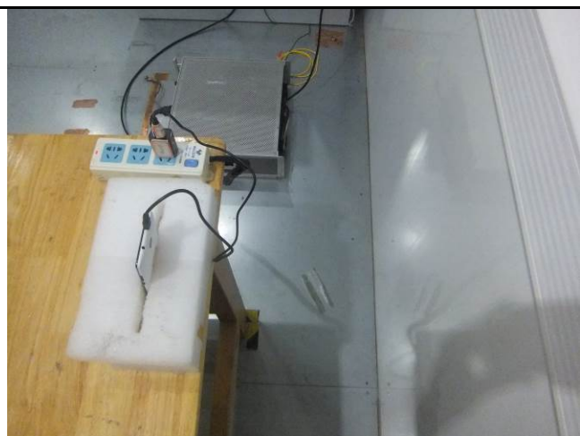
Conducted Emissions Test Setup Side View
