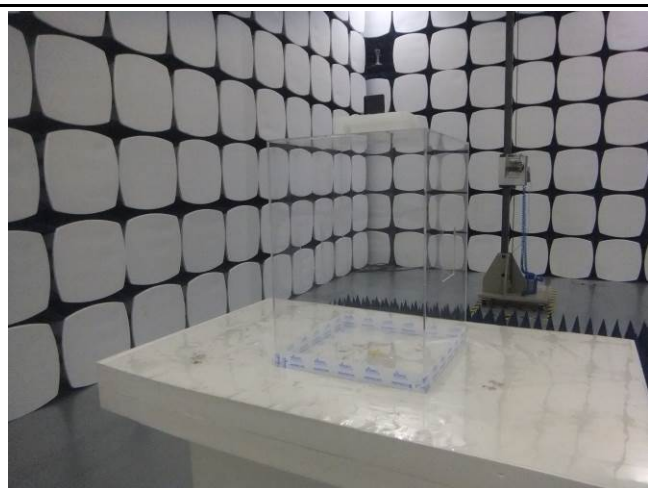
Radiated Spurious Emissions Test Setup Above 1GHz
