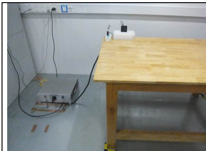
Conducted Emissions Test Setup Front View
