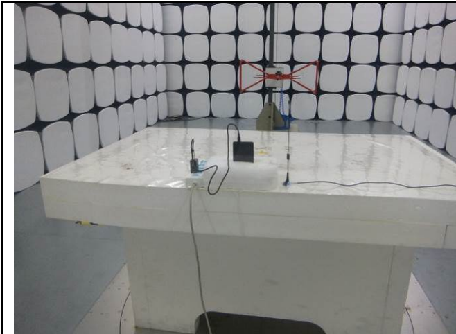
Radiated Spurious Emissions Test Setup Below 1GHz
