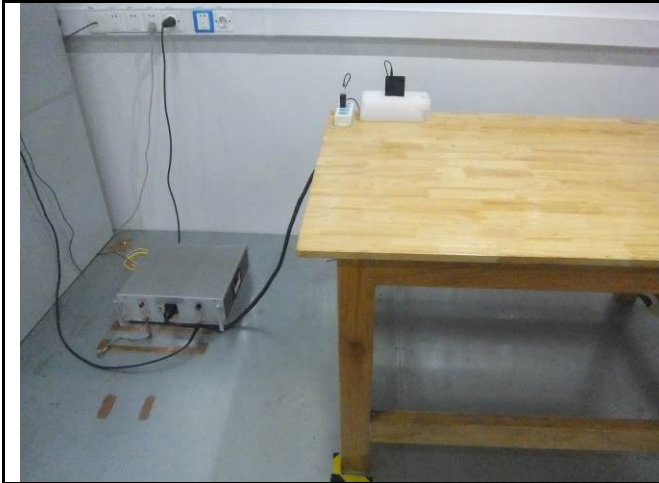
Conducted Emissions Test Setup Front View
