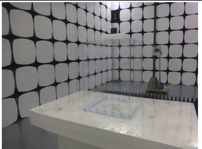
Radiated Spurious Emissions Test Setup Above 1GHz
