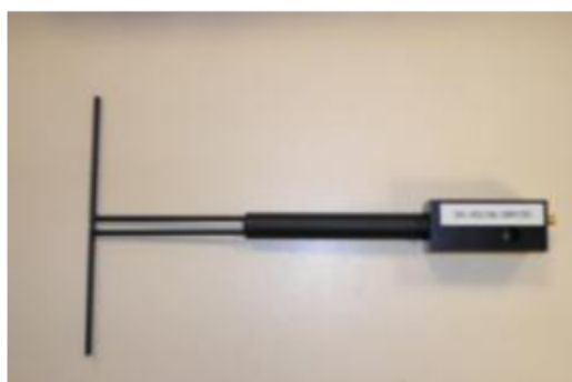
Figure 1 – Satimo COMOSAR Validation Dipole
