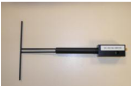
Figure 1 – Satimo COMOSAR Validation Dipole
