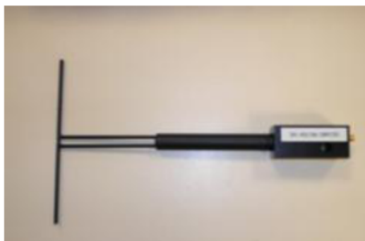
Figure 1 – Satimo COMOSAR Validation Dipole
