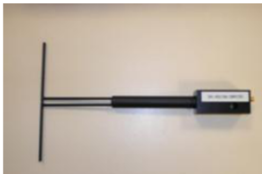
Figure 1 – Satimo COMOSAR Validation Dipole
