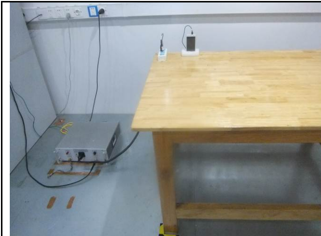
Conducted Emissions Test Setup Front View
