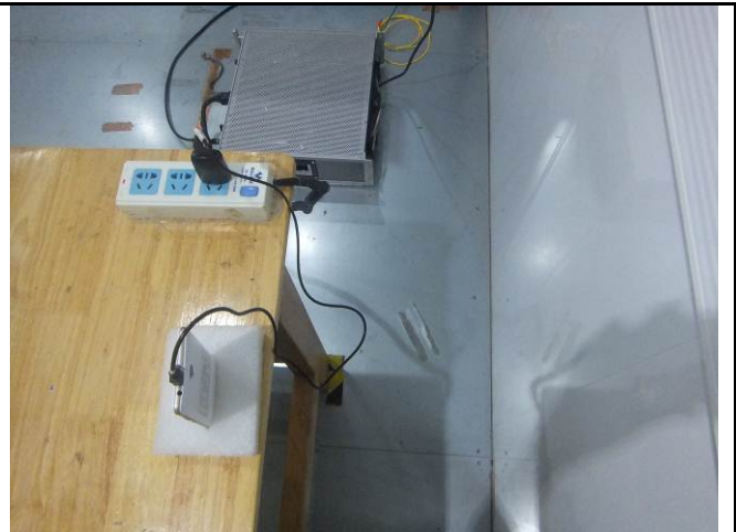
Conducted Emissions Test Setup Side View
