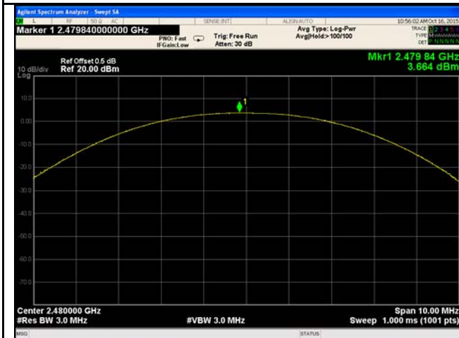
8DPSK Output power - High CH 2480
