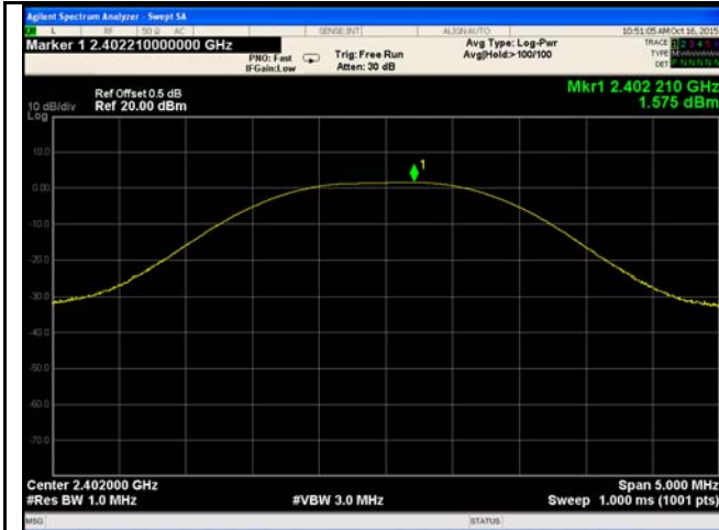
GFSK Output power - Low CH 2402
