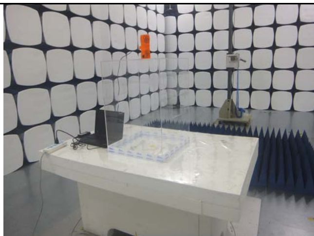
Radiated Spurious Emissions Test Setup Above 1GHz
