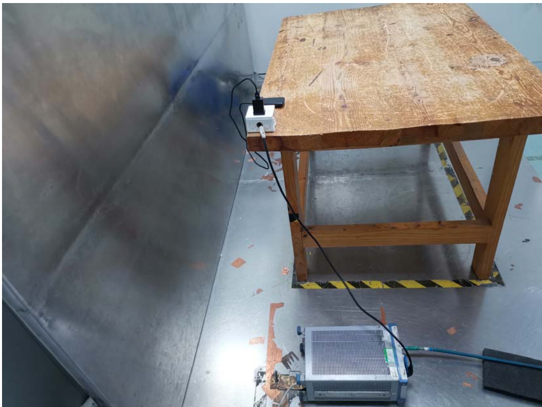
Conducted Emissions Side View
