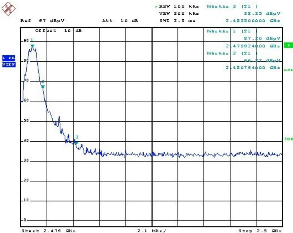
According to the page 15 of this report, the emission of the fundamental frequency 2480MHz is 87dBuV/m for peak level respectively. Based on the delta method, the emission at the bandedge, 2483.5MHz, is more than 40dB below the fundamental and 20dB bandwidth falls in the assigned band. It is deemed to comply with section 15.215. Besides, it is below the limit of 74dBuV/m and 54dBuV/m for peak and average level under 15.209. It is deemed to comply with section 15.249(d).
