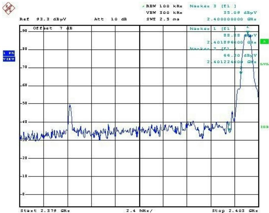
According to the page 15 of this report, the emission of the fundamental frequency 2402MHz is 88.1dBmV for peak level respectively. Based on the delta method, the emission at the bandedge, 2400MHz, is more than 40dB below the fundamental and 20dB bandwidth falls in assigned band. It is deemed to comply with section 15.215. Besides, it is below the limit of 74dBmV and 54dBmV for peak and average level under 15.209. It is deemed to comply with section 15.249(d).
