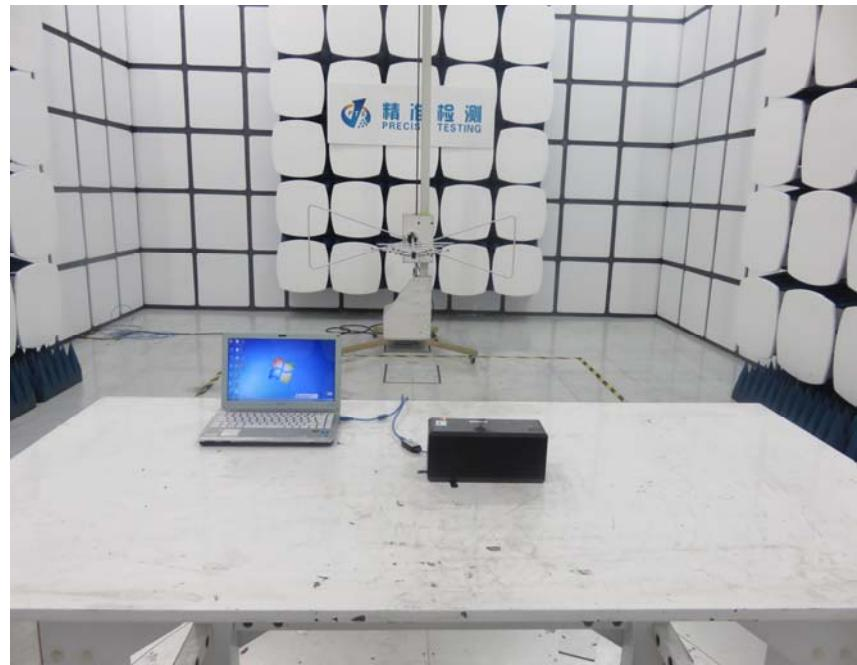
FCC RADIATED EMISSION ABOVE 1G TEST SETUP
