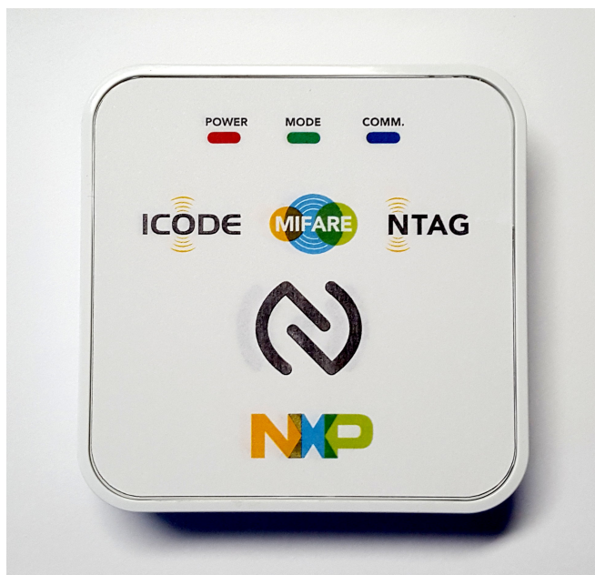
Figure 23. The top side of the reader CLRD730 with LEDs
