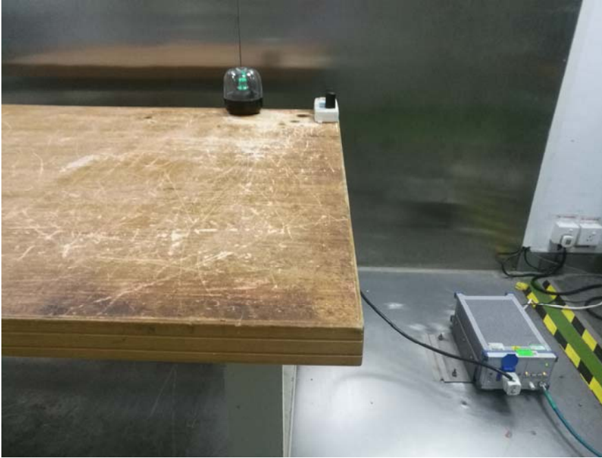
Conducted Emissions - Front View
