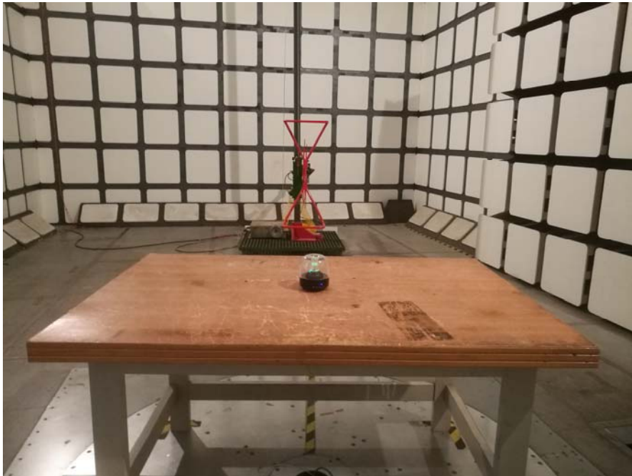
Radiated Emissions View (Below 1 GHz)
