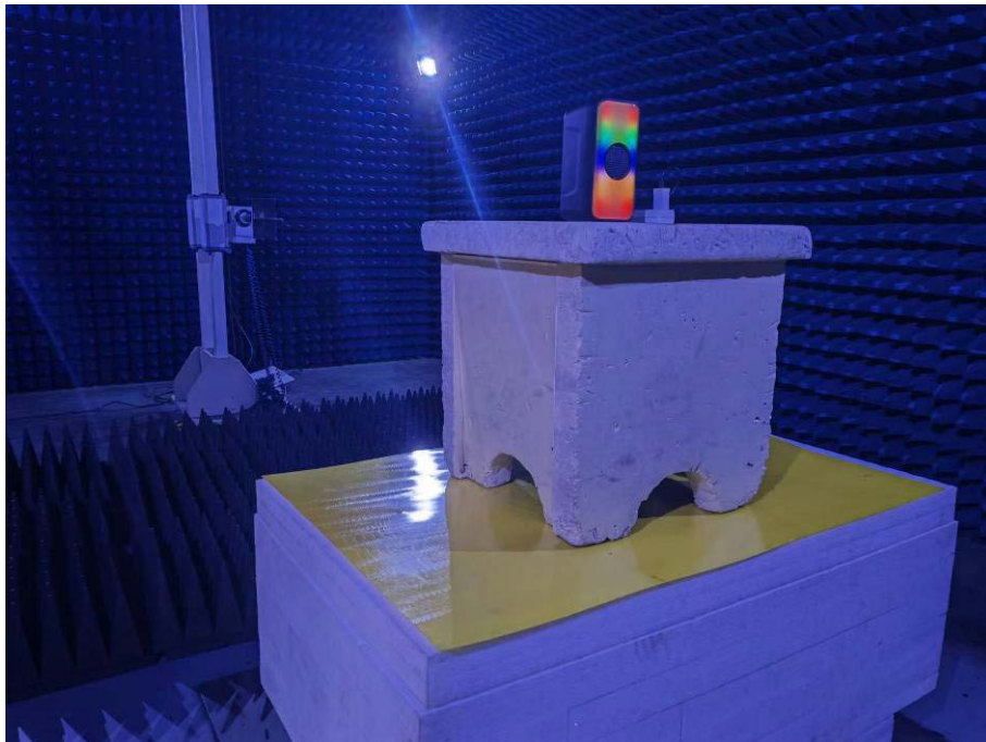
Photo of Radiated Emission Measurement Above 1GHz
