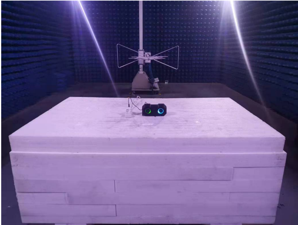
Photo of Radiated Emission Measurement (Above 1G)
