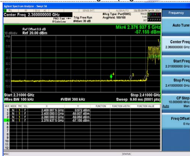
Left Band edge hopping on
