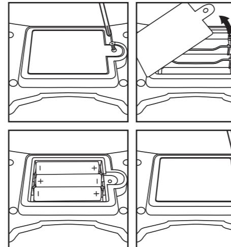
To install batteries into the Amphibious RC Car Remote, unscrew the screw on the battery box cover to open the cover. Insert 3 x "AAA" 1.5V batteries (Not Included) into the battery box. Batteries should be placed as shown on the diagram. Replace the battery box cover and tighten the screw.
