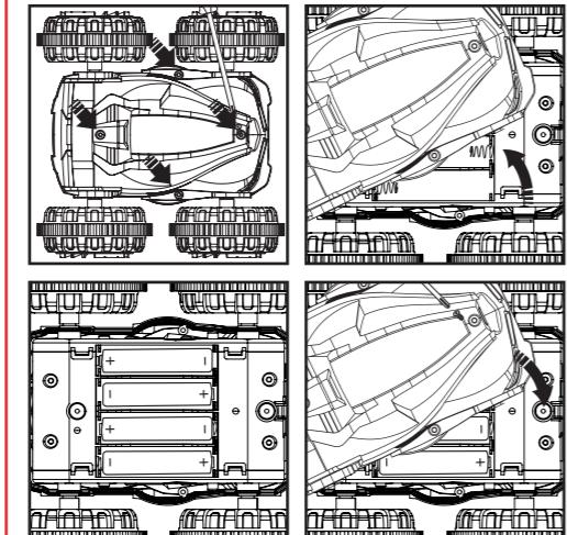
To install batteries into the Amphibious RC Car, unscrew the screws on the battery box cover to open the cover. Insert 4 x "AA" 1.5V batteries (Not Included) into the battery box. Batteries should be placed as shown on the diagram. Replace the battery box cover and tighten the screws.
