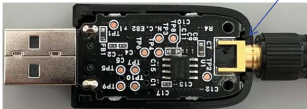
Wireless MCU on the PCB (Bottom)
