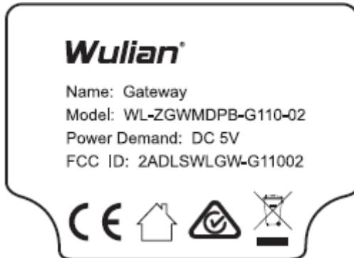
Specifications: Text is Black in color and justified. Labels are printed in indelible ink on permanent adhesive silk-screened onto the EUT or shall be affixed at a conspicuous location on the EUT.
