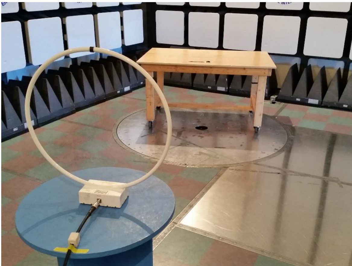
Figure 2 – Radiated Emissions Setup – Photo 1
