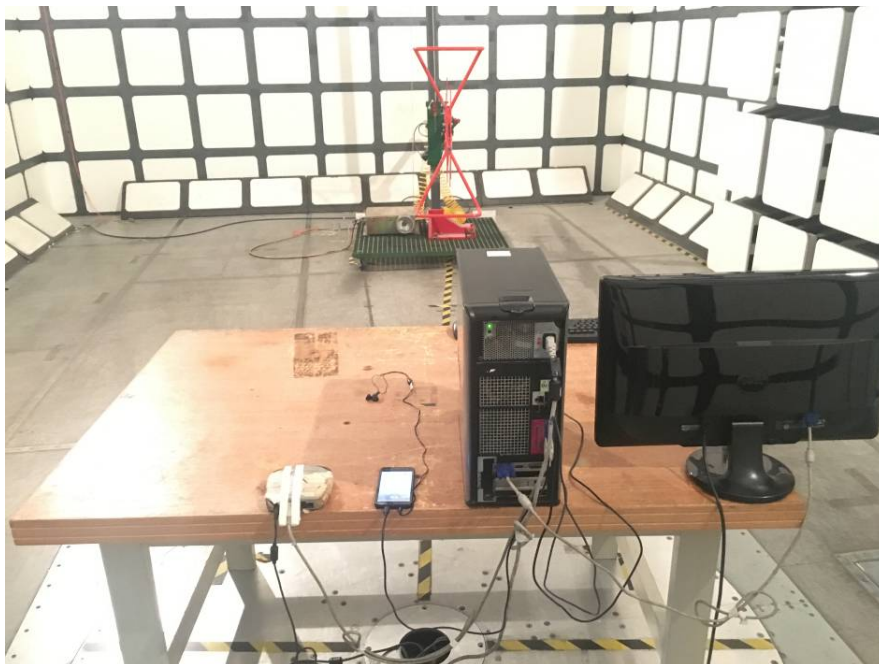
Radiated Emissions – Rear View (Below 1 GHz)
