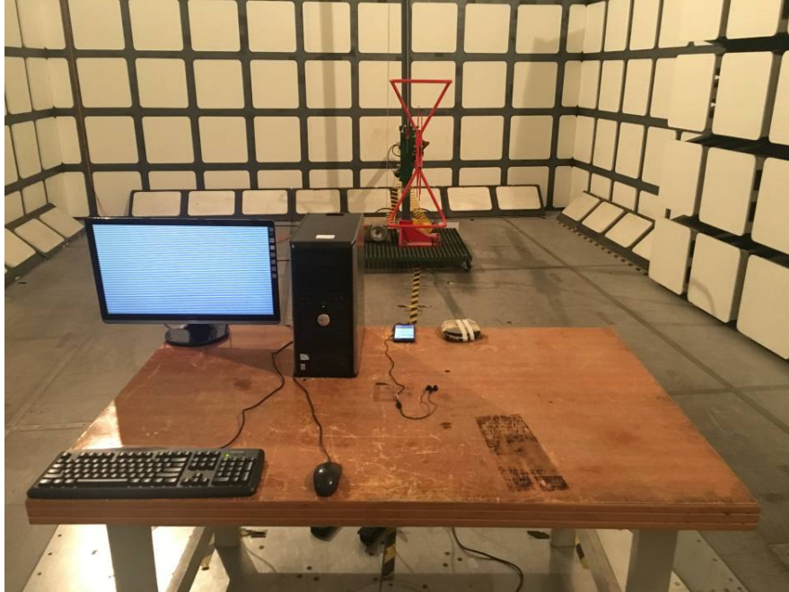
Radiated Emissions – Front View (Below 1 GHz)
