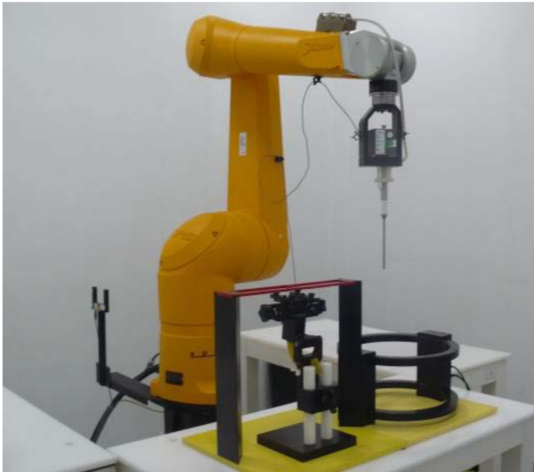
Picture 1: HAC T-Coil System Layout
