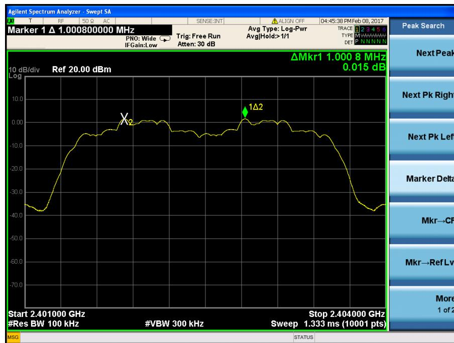
Channel Spacing (Middle CH=1MHz)
