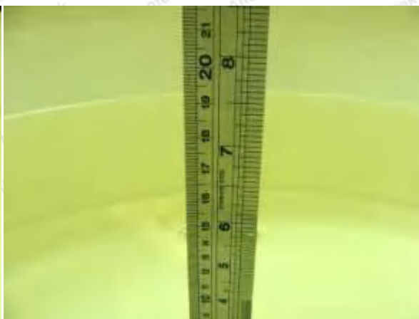
Photo of Liquid Height for Body SAR
