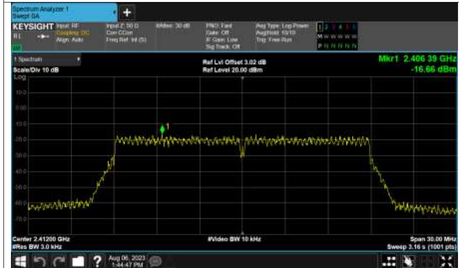
PSD NVNT n20 2437MHz Ant1
