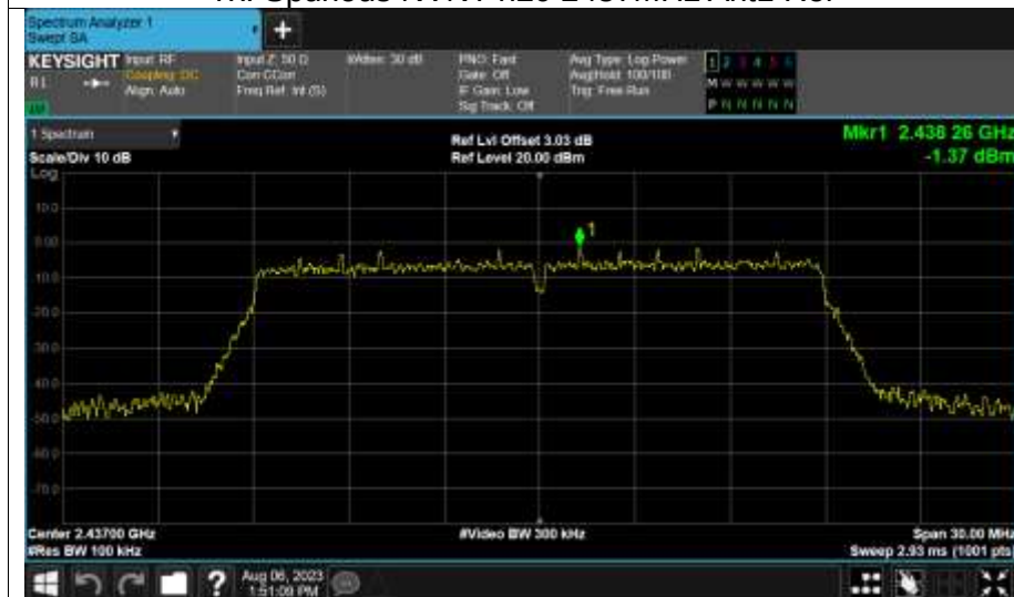
Tx. Spurious NVNT n20 2437MHz Ant1 Ref
