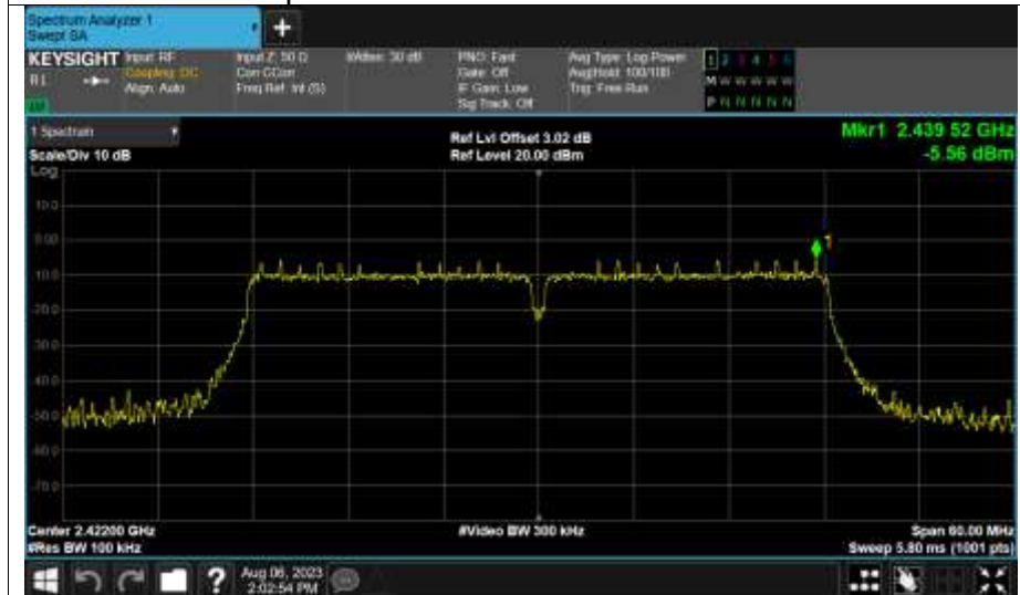
Tx. Spurious NVNT n40 2422MHz Ant1 Emission
