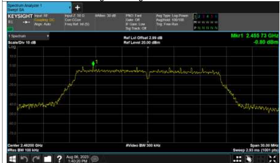
Band Edge NVNT g 2462MHz Ant1 Emission
