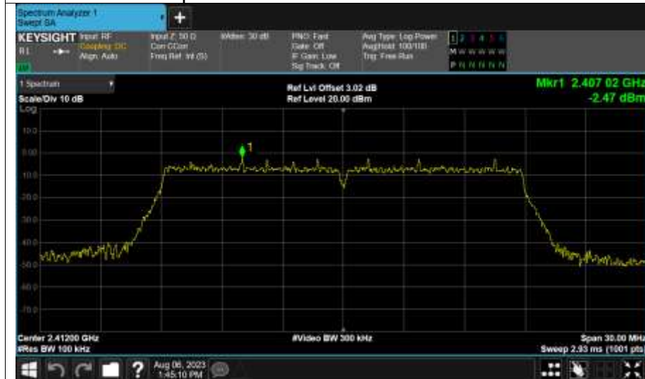
Tx. Spurious NVNT n20 2412MHz Ant1 Emission
