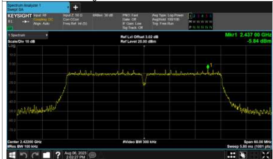
Band Edge NVNT n40 2422MHz Ant1 Emission
