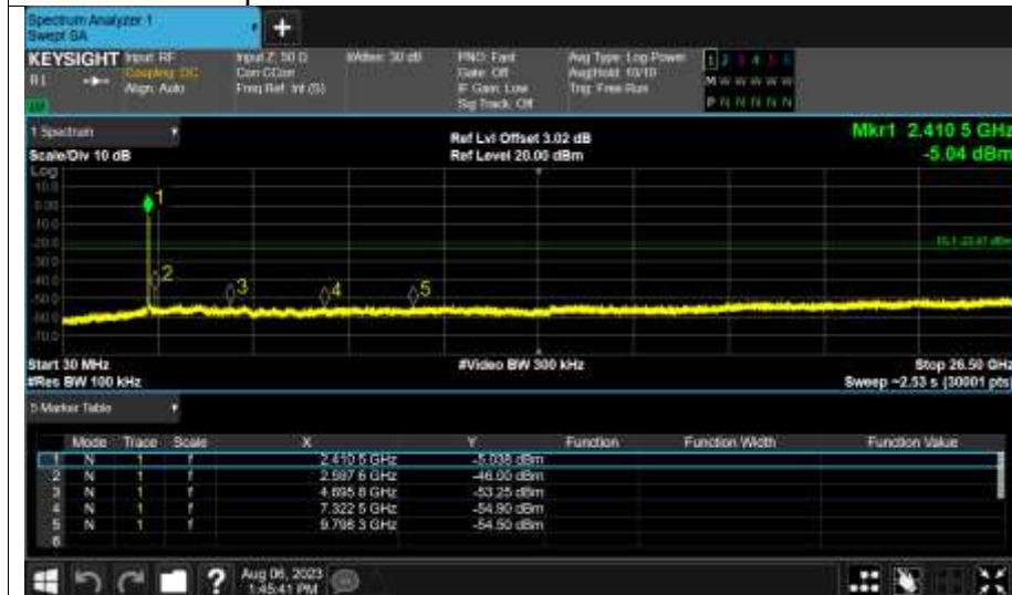
Tx. Spurious NVNT n20 2437MHz Ant1 Ref
