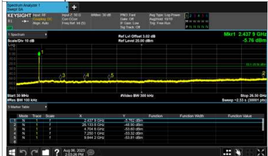
Tx. Spurious NVNT n40 2437MHz Ant1 Ref
