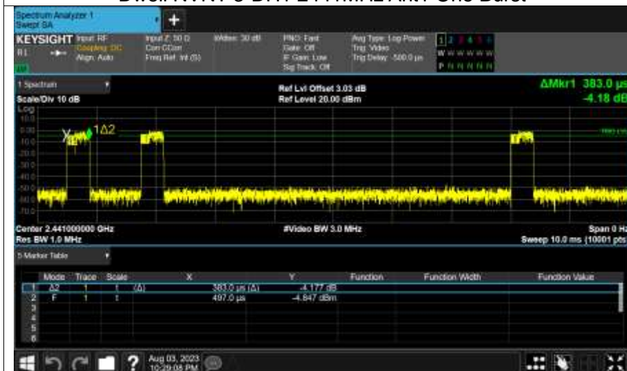
Dwell NVNT 3-DH1 2441MHz Ant1 Accumulated
