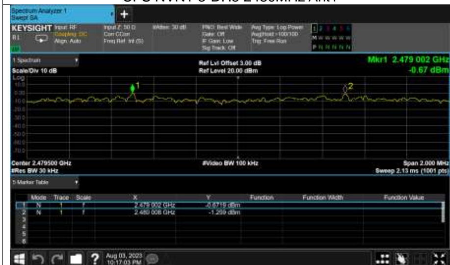
CFS NVNT 3-DH5 2480MHz Ant1
