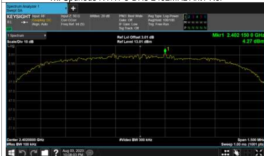
Tx. Spurious NVNT 3-DH5 2402MHz Ant1 Emission
