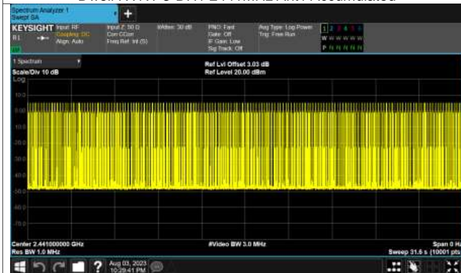
Dwell NVNT 3-DH3 2441MHz Ant1 One Burst
