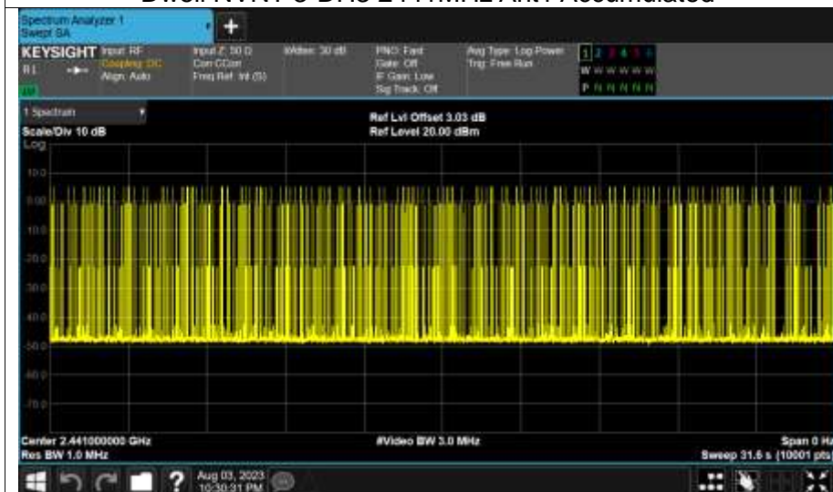
Dwell NVNT 3-DH5 2441MHz Ant1 One Burst
