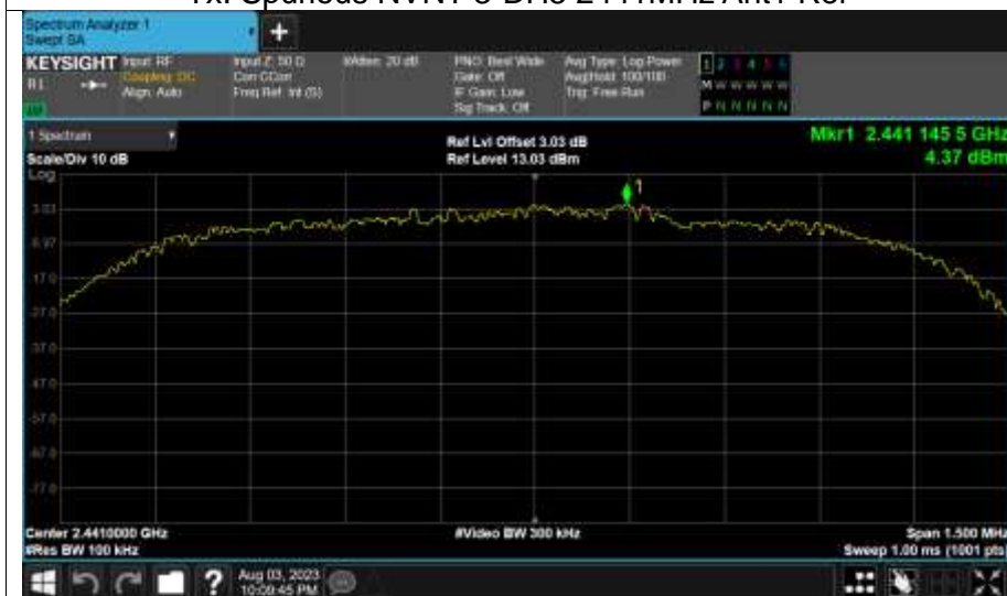
Tx. Spurious NVNT 3-DH5 2441MHz Ant1 Ref
