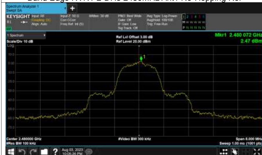
Band Edge NVNT 2-DH5 2480MHz Ant1 No-Hopping Emission
