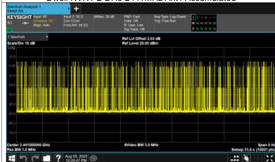
Dwell NVNT 2-DH5 2441MHz Ant1 Accumulated
