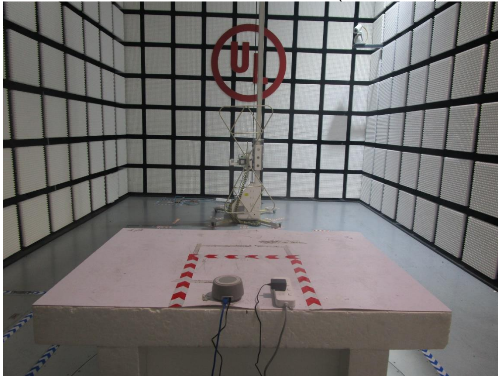
RADIATED RF MEASUREMENT SETUP (Below 30MHz)
